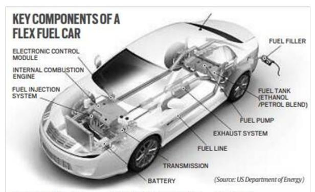
BATTERY: The battery provides electricity to start the engine and power vehicle electronics/ accessories
