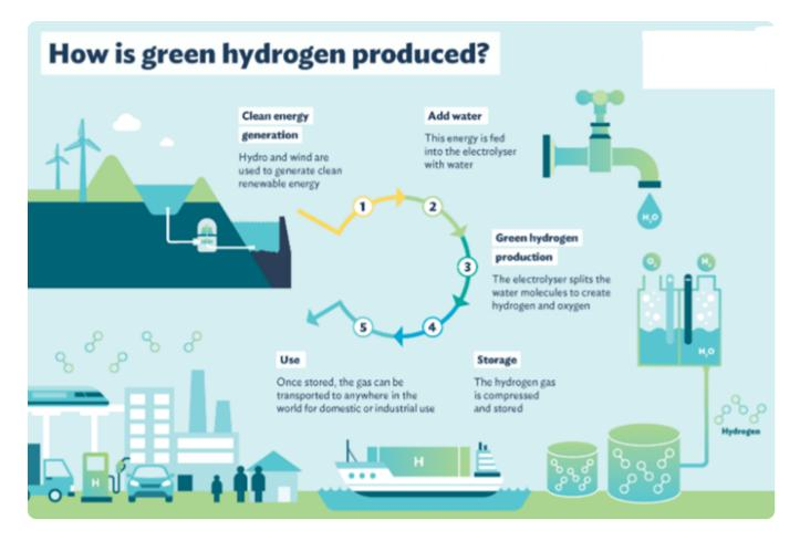
Green hydrogen refers to **hydrogen that is produced from the electrolysis of water** — splitting it into hydrogen and oxygen — using an electrolyser powered by renewable energy.
