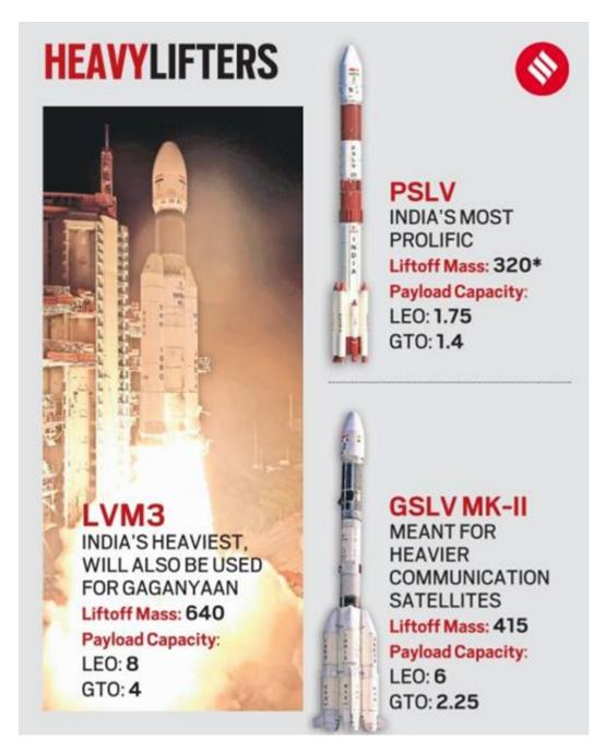
LVM3 is the culmination of more than three decades of efforts to indigenously develop a rocket that can carry heavier payloads, or venture much deeper into space. These requirements not only result in a massive increase in the size of the rocket, but also necessitate a change in the engines and the kind of fuel being used.
